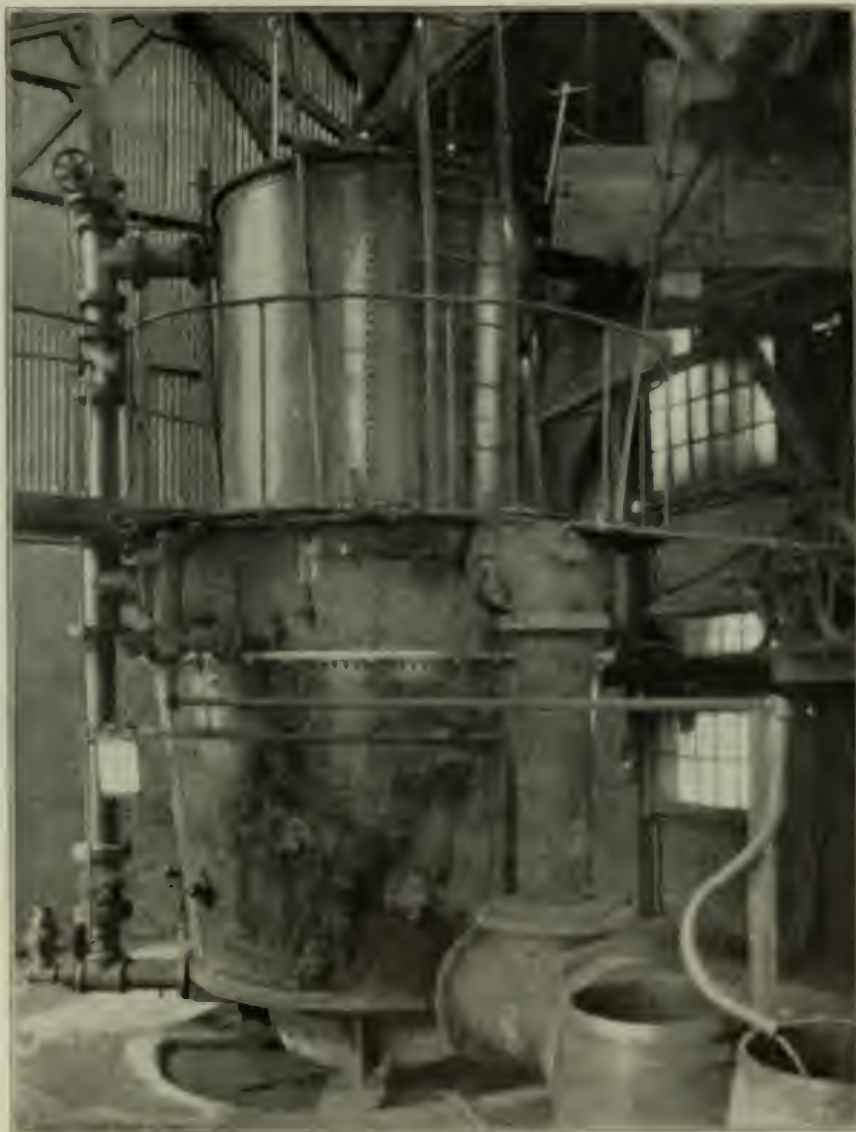
FIG. 1. 175 HORSEPOWER WASHINGTON UNIVERSITY GAS PRODUCER TYPE DE HOUSE BUILT AT EAST COTTON.
